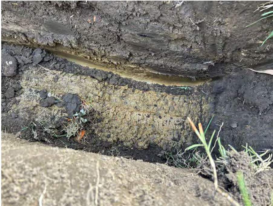
Image 9.1.2.2 Photograph of fill and natural profile from TP16.
