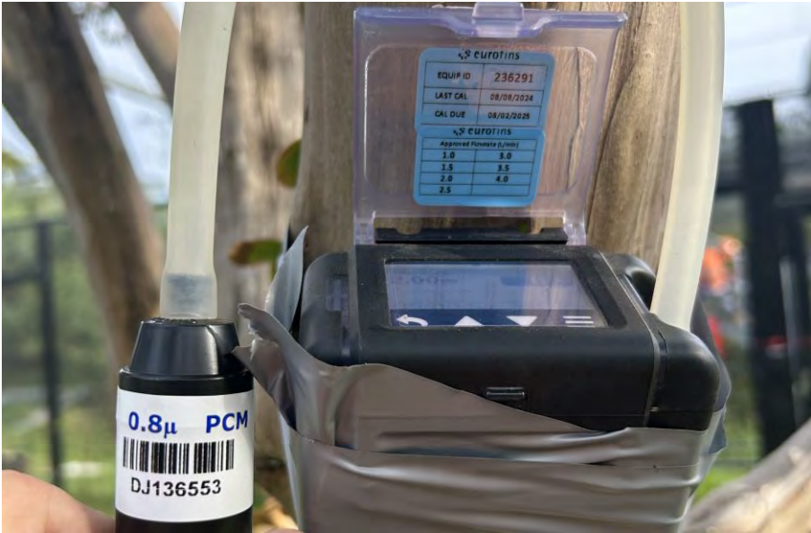
Image 9.1.1.2 Photograph of air monitor set up.
